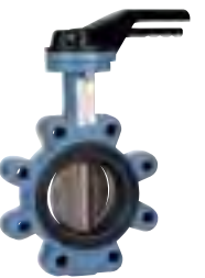
1162 - Disc CF8M up to DN100, Disc GGG50 epoxy coated above / Seat NBR TS: -10°C/+90°C.
