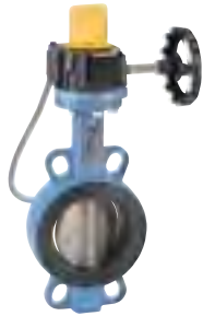
1144 - Disc CF8M up to DN100, Disc GGG50 epoxy coated above / Seat EPDM For fire network - FM approved - With gearbox & limit switches - TS: -10°C/+110°C.
