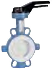
1155 - Disc CF8M + TEFLON® / Seat TEFLON® with silicone liner TS: -25°C/+200°C.
