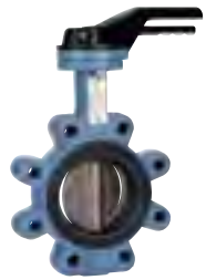
1160 - Disc CF8M up to DN100, Disc GGG50 epoxy coated from DN125 to DN300, Disc GGG50 rilsan coated above / Seat EPDM TS: -10°C/+110°C.
