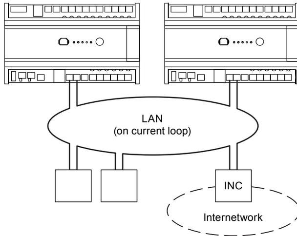
*Note: In this configuration IQ4E cannot join a Trend LAN on Ethernet. However, access by IP is still possible.*
