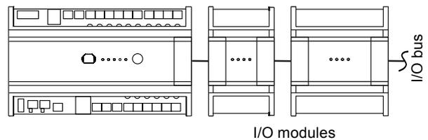
Several IQ4E variants are available to provide support for differing numbers of I/O channels up to a maximum of 192 (16 onboard, 176 on I/O bus) (see 'Order Codes' on page 10).
