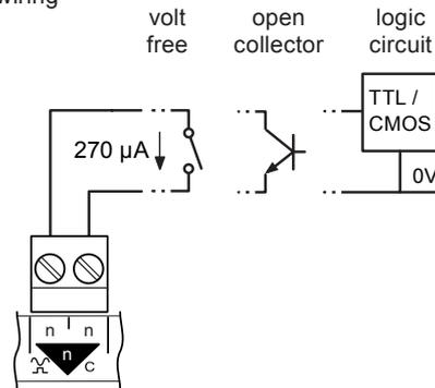
The volt free contact has a nominal wetting current of 270 μA. The input is ON when the contact is closed.
