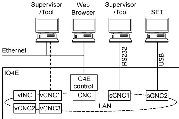
**Default CNC Addressing:** The IQ4E device (outstation) address is factory-set (in the Address module) as follows:
